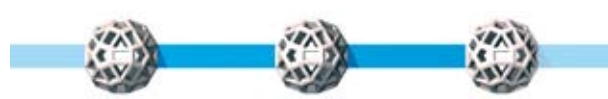
A line of equally spaced balls is like a one-dimensional lattice. Notice that all the balls are oriented the same.
